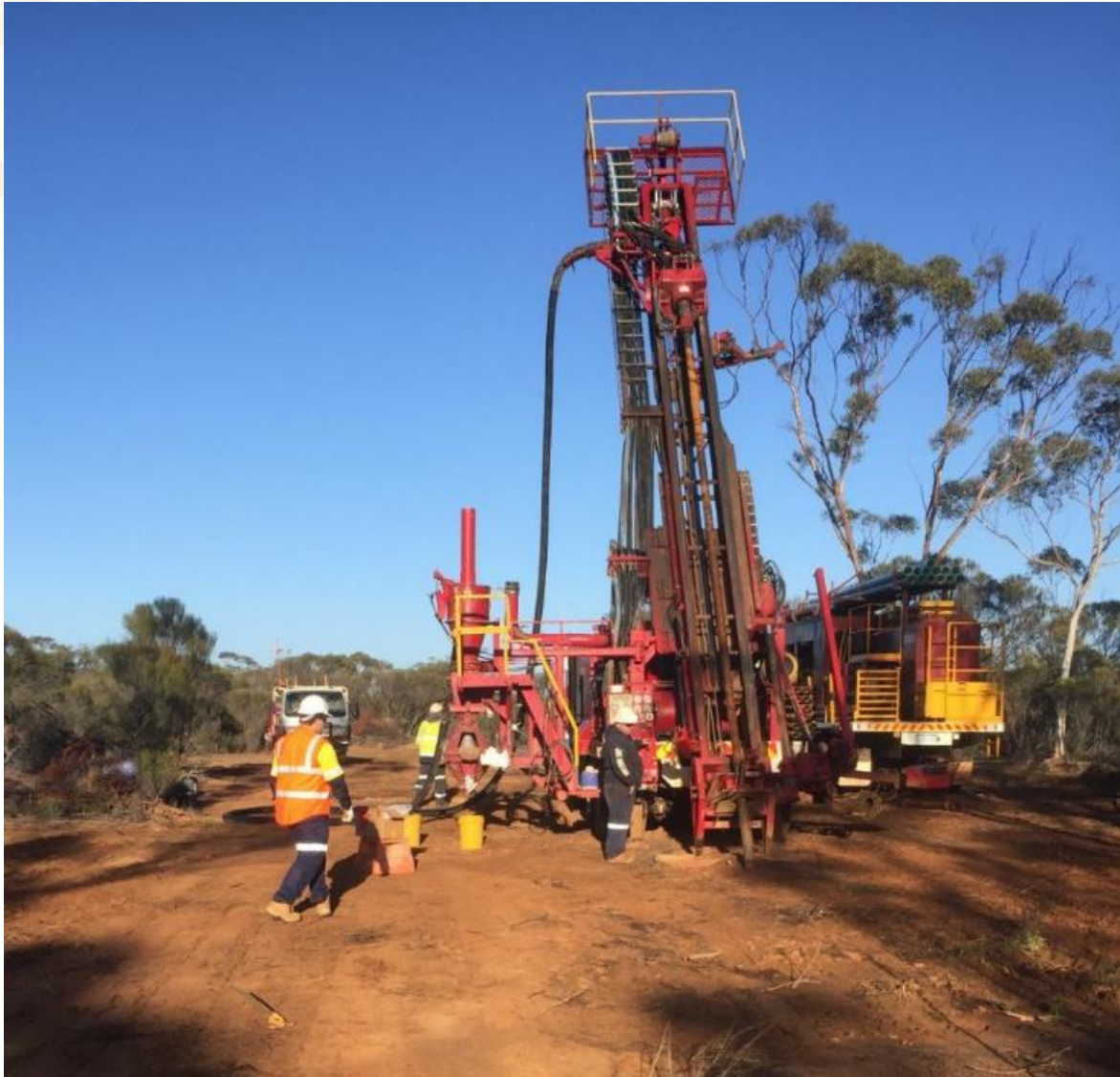
Figure 1: RC drill rig in operation at the Glendower gold prospect
